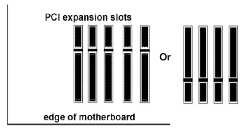
Insert the MegaRAID Express 500 card in a PCI slot as shown below:
